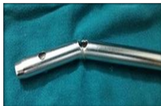
Figure 4: Shows nail broke at site of nicking
