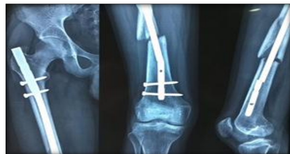
Figure 1: shows broken femur nail at proximal screw slot of distal locking screws
